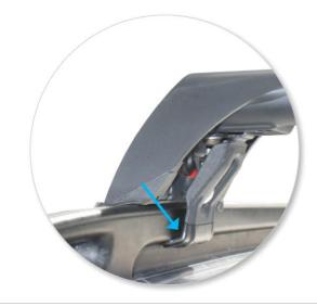
• Ensure the clamp engages correctly on inside of roof rail.
