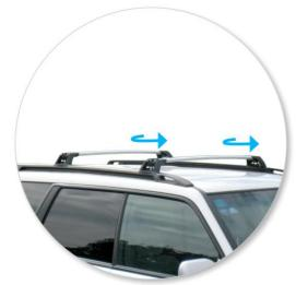
Place crossbars back onto vehicle roof by placing one end of crossbar on the rail and swing the other into previously marked position.
