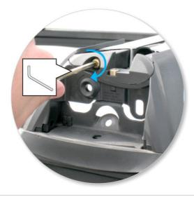
• Tighten adjusting screw to 5 Nm.
