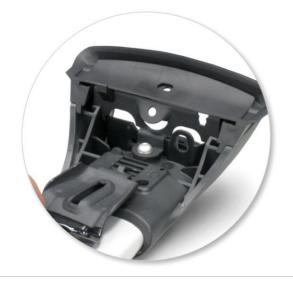
Remove crossbar off vehicle and turn upside down. Select metal clamp and fit small tongue into position 2 marked on the leg.
