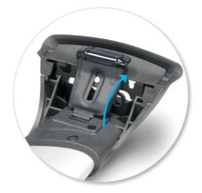
Swing clamp towards metal loadplate and check clamp tongue is engaged into position.
