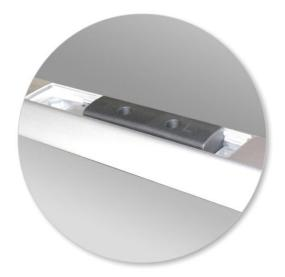
Select plastic packer blocks from fitting kit and insert into fixed-points. Blocks have L & R which should be read from beside vehicle.
