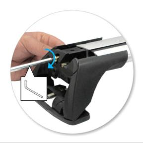
• Tighten adjusting screw to 5 Nm.
