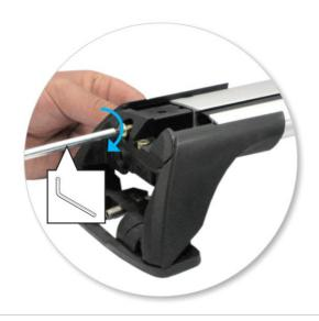
• Tighten adjusting screw to 5 Nm.
