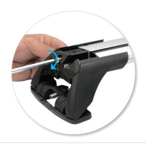
• Tighten adjusting screw to 5 Nm.
